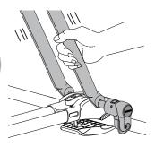
• PERIODICALLY CHECK THAT KNOBS ARE ADEQUATELY TIGHTENED.
