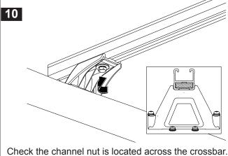
Using the security allen key provided tighten legs to brackets then the brackets to each other until secure. Recommended tightening torque 3-4N/m. DO NOT OVER TIGHTEN.
