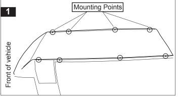
Hook the inner (smaller) bracket under the mounting point.
