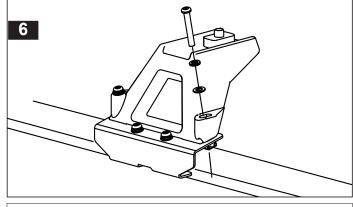
Place the crossbar onto the support legs. Push the crossbar attachment bolt up and turn the bolt so that the channel nut is located fully across the crossbar. Finger tighten the crossbar attachment bolts.
