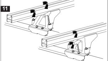
Insert the crossbar rubber buffer strip into the top of the crossbar. Insert end caps into the ends of the crossbar using rubber mallet. Check all attachment bolts and screws are secure after fitment.
