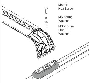
Remove rubber covers over threads on the factory rails. Fixture points are located on both rails facing inward. Install bracket assembly.
