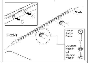
When crossbars are not in use, remove and install the cover plates as shown.
