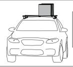
75kg/165lbs load rating (Urban road) 50kg/110lbs load rating (Off road - 75kg / 1.5)
