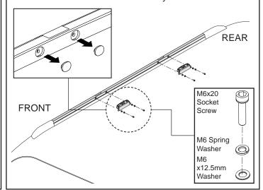
Fix the completed crossbars to the vehicle with an M6x16mm hex, M6 spring and flat washer (RVH shown as example only).
