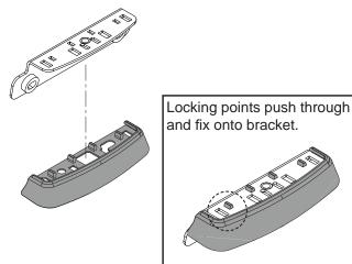
Remove rubber covers over threads on the factory rails. Fixture points are located on both rails facing inward. Install bracket assembly.
