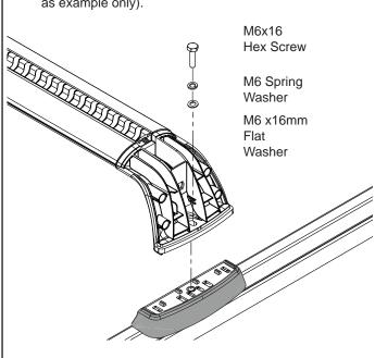
When crossbars are not in use, remove and install the cover plates as shown.
