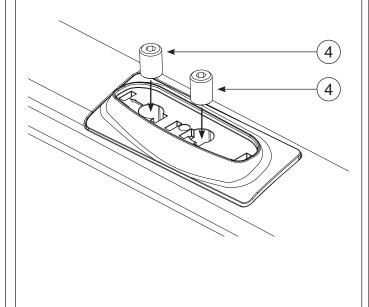
Fix the crossbars to the vehicle using the M6 x 30mm hex setscrew, M6 spring washer and flat washer provided as per corresponding instructions. When crossbars are not in use, remove and install the mount point cover plates as shown.
