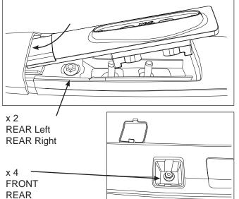
Fasten all four base pads with M8 tube nuts. 3-4 Nm (2-3 lb/ft). Use 5mm Allen key supplied.
