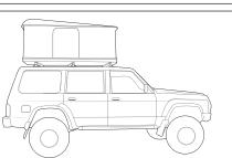
When these roof racks are to be used on a vehicle that is driven off sealed roads the maximum load rating must be divided by 1.5.
