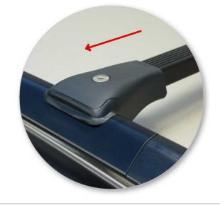
Pull legs out evenly until both rubber gasket seal on roof rail.
