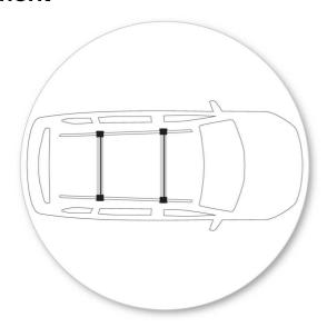
This product has two different bar lengths. The longer bar should be used on the front of the vehicle and the shorter bar used on the rear.
