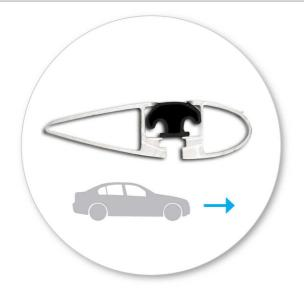
Ensure the roof rack face towards the front of vehicle.
