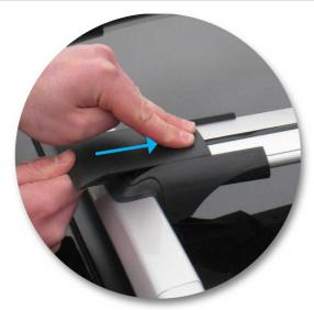
Slide Hex Key back into position into one of the roof rack legs.
