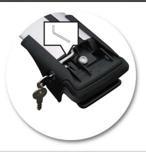
• Locate the Hex Key in one of the roof rack legs.
