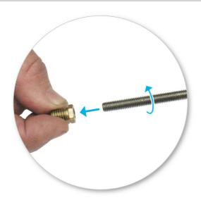
Select four grubscrews and assemble them into the adaptor using 3 mm (1/8") Hex Key.
