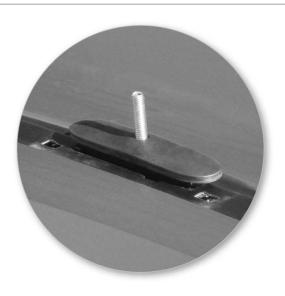
Place load support over grubscrew as shown.
