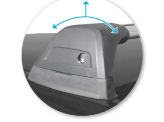
CAUTION: Recheck all fasteners immediately after a load is applied to the crossbars. Regularly check screws are tight.
