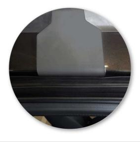
The rubber seal must be peeled back from the vehicle body to allow the clamp to be inserted between the vehicle body and the rubber seal.
