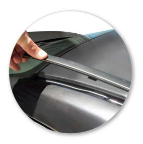
Lift and pull ditch moulding back towards you and remove from the vehicle.
