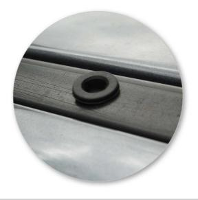
If crossbars are removed, please install the rubber plugs into the ditch moulding. CAUTION: Recheck all fasteners immediately after a load is applied to the crossbars.
