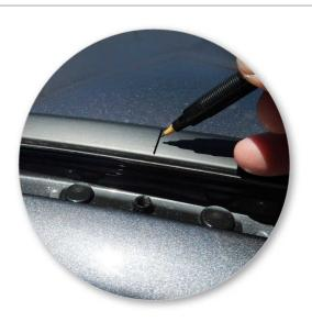
Mark a reference point for the front and rear mounting points with a pen as shown.
