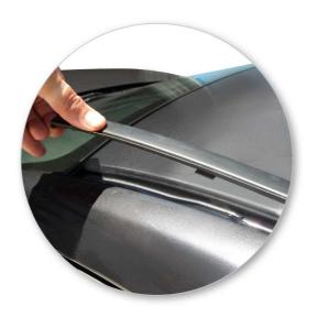
Re-install rubber ditch mould back into roof channel and click into place.
