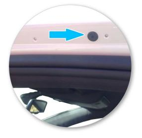
Locate vehicle's fixed points for the front bar.
