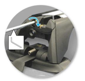
Tighten adjusting screw to 3 Nm (2.2 ft lb) hand tight.
