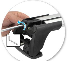
Use hex screwdriver to reverse adjusting screw 10 turns.
