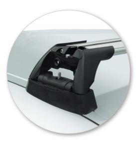
Place crossbars on pads ensuring the pads fit into the holes underneath the foot and the grubscrew pass through the hole in the foot.
