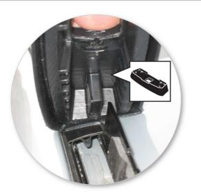
Ensure the fixed-point covers sit vertically in the recess in the pads.
