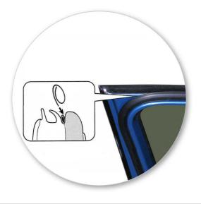
• Ensure door seal positioned as shown.
