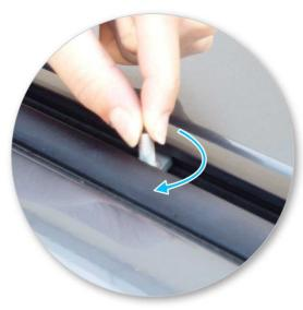
Rotate bolt clockwise so it engages in place in the centre of track.
