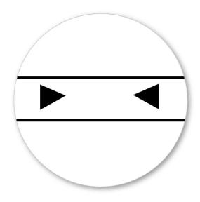
Place the clamp between the marks on the body rubber
